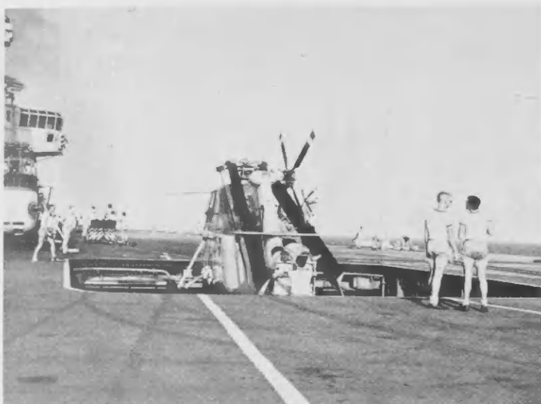
MOVEMENT OF aircraft from the flight deck to the hangar deck, below the flight deck, is done by two elevators at either end of the ship. When up, the platform of the elevator becomes a solid part of the flight deck. The carrier's detection and navigation gear towers above the deck.
